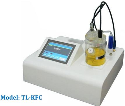
TOPLAB INDIA'S **Coulometric Karl Fischer titration** is the most reliable method to detect moisture at trace level for different substances, which was utilized successfully by **TL-KFC** Trace Moisture Analyzer.
